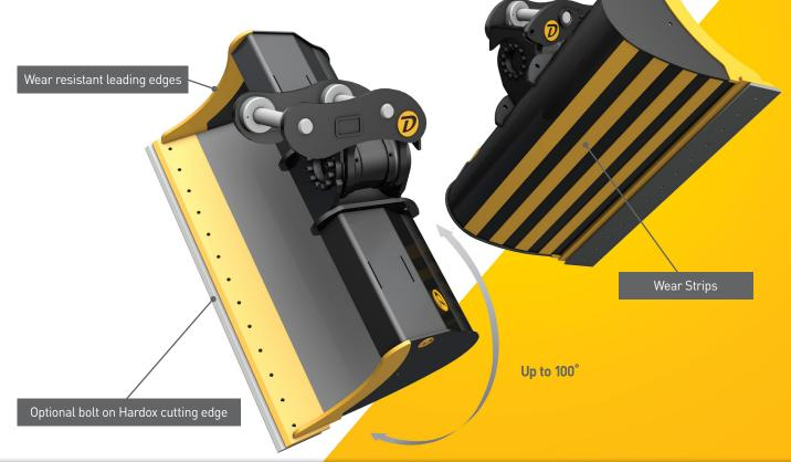
The BTA range of buckets are manufactured from medium and high tensile steel which is wear resistant to optimise strength and weight. A wide selection of widths are available and wear strips are standard on all models above 5.5 tonne. A reversible bolt on cutting edge is optional. Custom built designs are also available on request.
