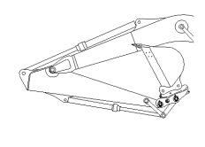
The installation of a quick coupler effectively lengthens the reach of your excavator's dipper arm. This may enable various attachments to come into contact with the boom set and operator's cabin. Operators must be aware of this and take appropriate care.
