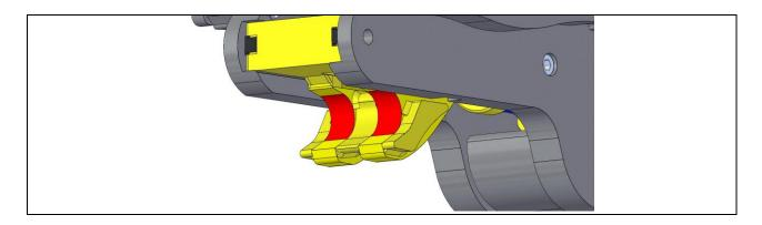
There are three wear areas that could be causing contact. It may be one area that is worn excessively or any combination of all three areas. All three areas should be checked and rectified if the below wear limits are exceeded.
