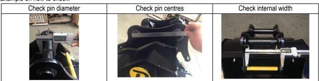
Note, Internal width should not exceed the width of the coupler more than 4mm per side, If coupler is used on Under cutters, rock saws or any other attachment which has a significant side load the coupler MUST be a tight fit.
