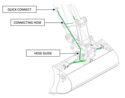
To establish the correct hose lengths, crowd the tilt bucket to each extreme and fully tilt each way to establish maximum hose length required. Take care when crowding back and tilting the opposite direction to ensure excess hose rolls up and does not foul on anything. The use of kevlar sleeves or "spaghetti" armouring is strongly recommended.
